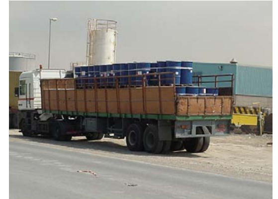
Unsafe Securing Arrangement
